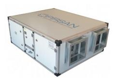
With the PHRV series heat recovery devices, it is aimed to keep the indoor air quality at comfort levels. With high efficiency plate heat exchangers, heat transfer is carried out without mixing fresh air and exhaust air, and the heat left by the exhaust air is loaded and blown into the space.
