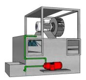
PSF series water filtration plants; It is designed for washing the air in enterprises with oily and sooty exhaust air such as industrial kitchens, restaurants and factories.
